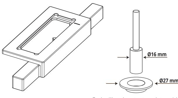
End mill and router template guide
