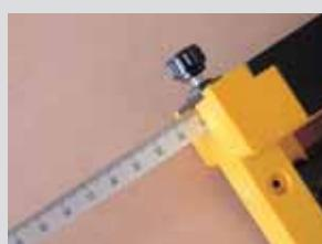
**2** • The millimetric rod allows the correct positioning of the jigs on the frames and on the doors.
