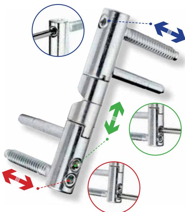
This high quality hinge, as well as being adjustable in three directions, also has a lifting action: **whilst the door is being opened, it lifts up by 5 mm.** It is therefore particularly suitable for wide and heavy doors and old uneven floors or for going over carpets and rugs, fully demonstrating its qualities of efficiency and precision.
