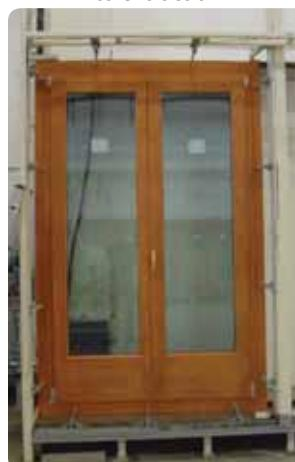
Test for resistance to water and wind
