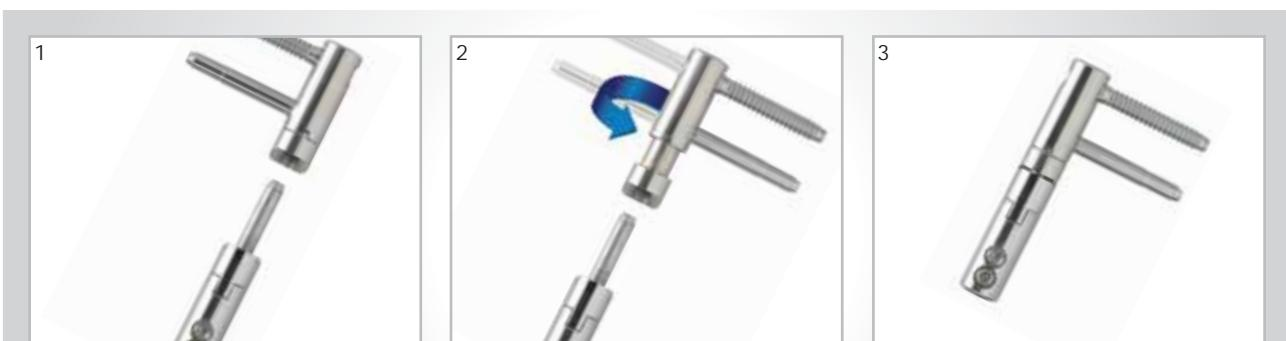
**1/2/3** - Acting on the upper part of the hinge, the female part, it is possible to change the direction of the hinge, from right to left and vice versa. It is sufficient to lift a few millimeters the movable part of the female hinge and rotate 180° to obtain a right or a left hinge.
